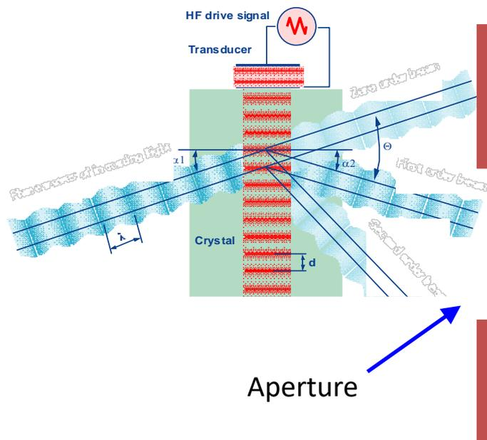
Figure 6: Schematic of a acousto-optic modulator.
