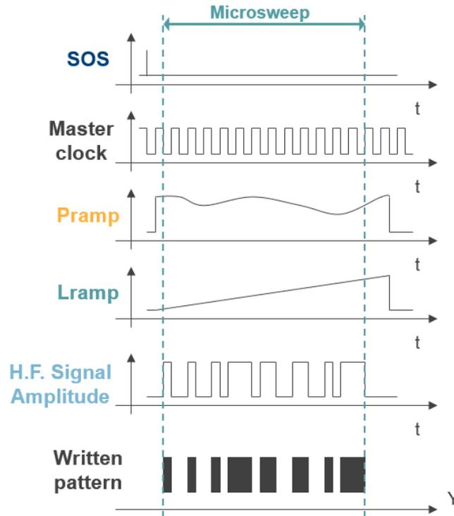
Figure 4: The synchronisation of an external event is used to localise the subsequent patterning.
