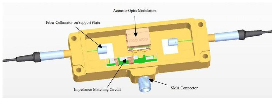
Figure 7: Example of the commercial acousto-optic modulator.
