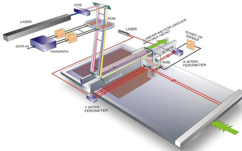
Figure 3: The pattern generation design is a raster scan system with acousto-optic deflection and modulation of the exposure laser.
