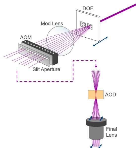
Figure 9: Schematic of the situation of the AOD in connection to the DOE and AOM.
