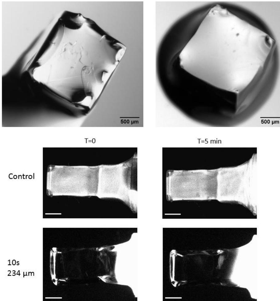
Figure 14: Top: examples of polymerized cubes of GelMa-PEGDA (left) and PN-PEGLink (right). Bottom: method to determine the 3D shape of the polymerized hydrogel regions by dissolving FITC-dextran in the FEP-cuvette after polymerization.
