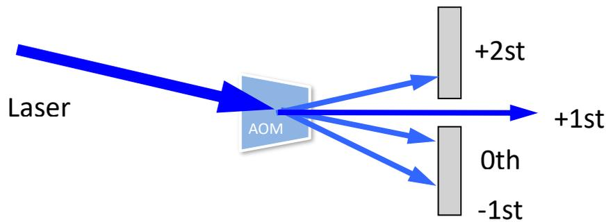
Figure 8: Amplification of the first order beam in the AOM.
