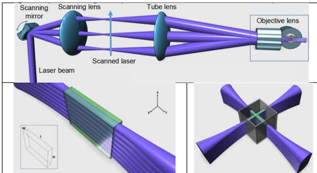
Figure 2. (a) Scheme of the light-sheet generation, (b) light-sheet size parameters and (c) 90° crossed set-up.
