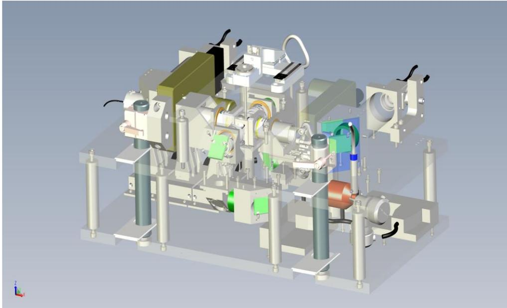
Figure 10: Overview of the first-iteration double-side LSFM Bioprinter realized for BRIGHTER.
