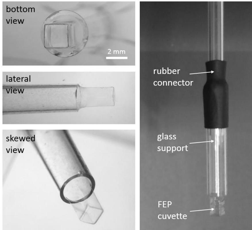
Figure 12: Optical set-up of the LSMF Bioprinter realized for BRIGHTER.
