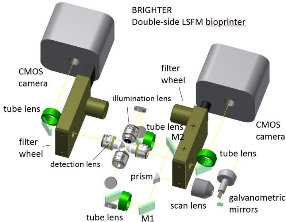
Figure 11: Optical set-up of the LSFM Bioprinter realized for BRIGHTEr.
